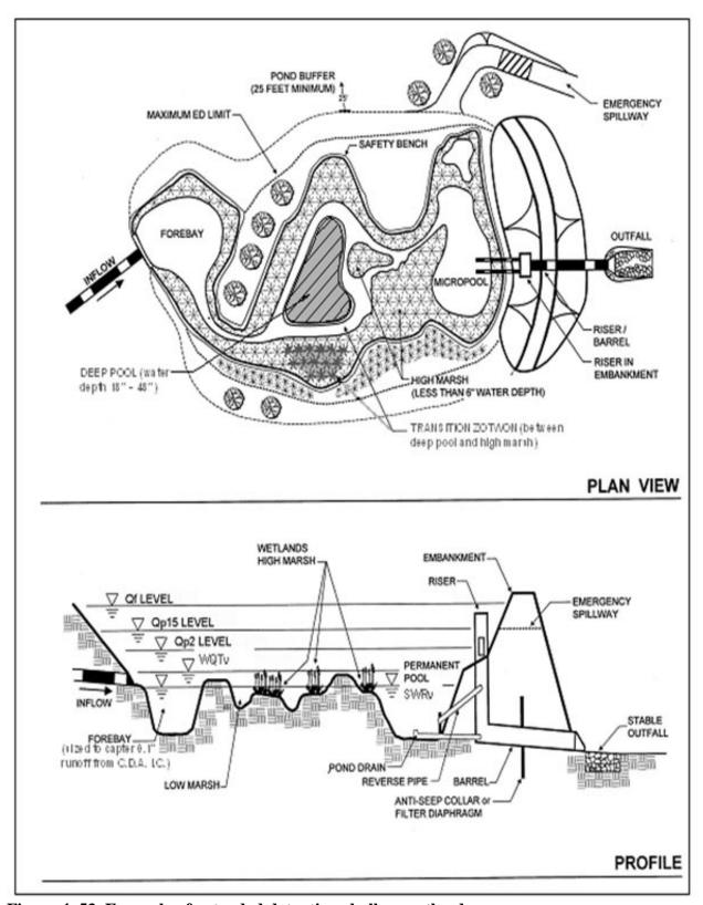
Figure 4. 53 Example of extended detention shallow wetland.
