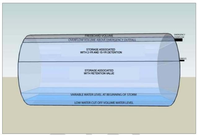
Figure 4.30. Incremental design volumes associated with cistern sizing.
