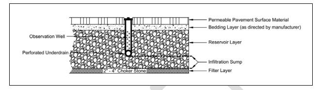
Figure 4.13. Cross-section of an enhanced permeable pavement design with an underdrain.
