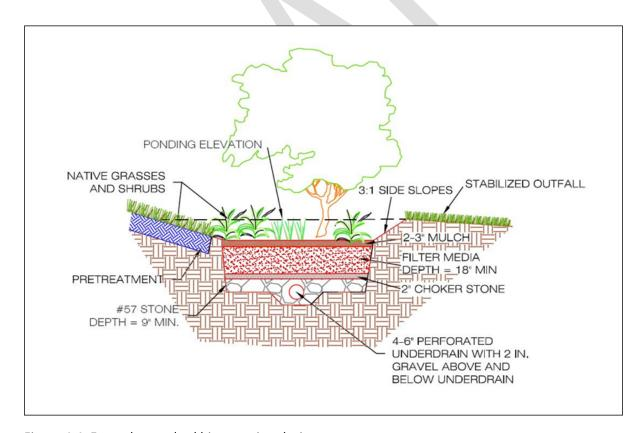
Figure 4.4. Example standard bioretention design.
