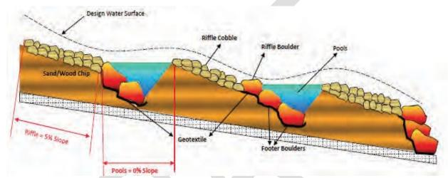
Figure 4.37. Example of Regenerative Stormwater Conveyance (O-4).
