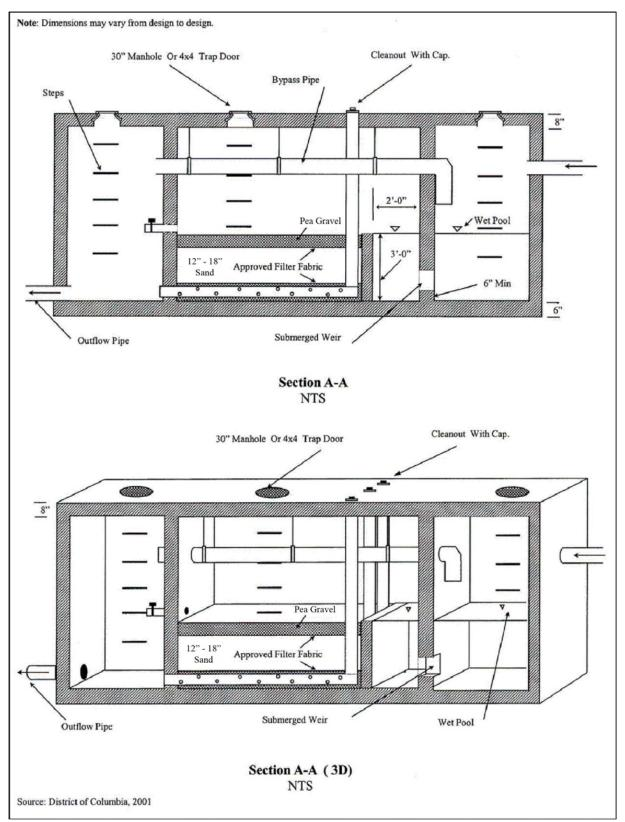
Figure 4.41. Example of a three-chamber underground sand filter (F-3) for separate sewer areas. Part B. Note: material specifications are indicated in Table 4.44.
