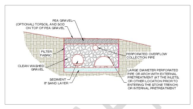
Figure 4.18. Example design of an infiltration practice with supplemental pipe storage.
