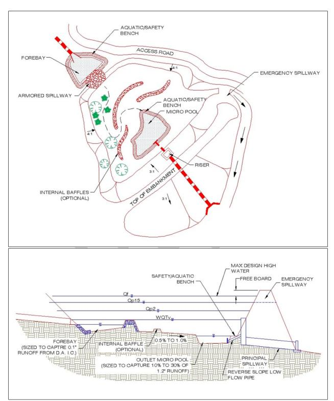
Figure 4. 51 Typical extended detention pond (C-3) details.
