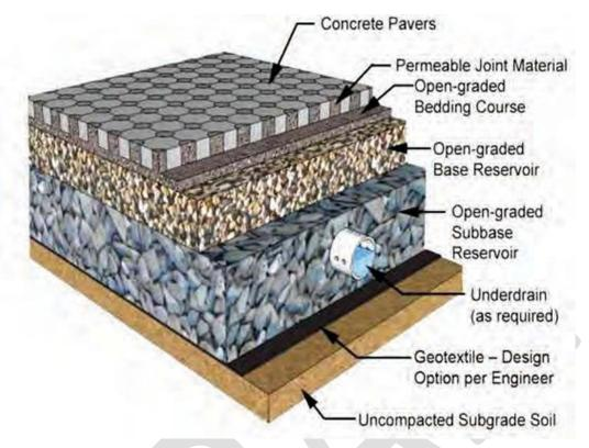
Figure 4.11. Cross-section of permeable pavement (source: ICPI).
