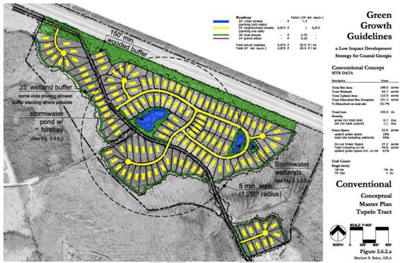
Figure 2.3. Conventional Site Design (source: Merrill et al., 2006).
