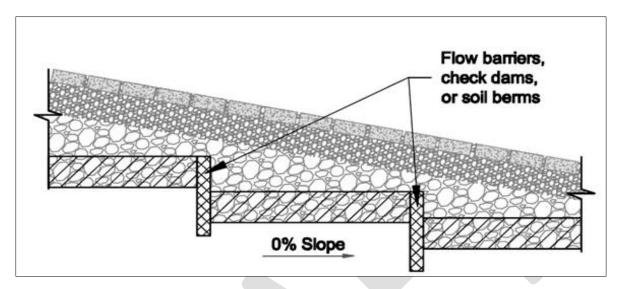
Figure 4.15. Use of flow barriers to encourage infiltration on sloped sites.
