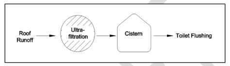
Figure 2. Example 2 treatment schematic.
