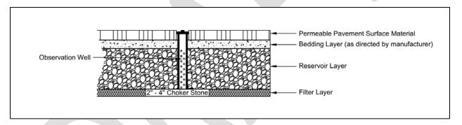
Figure 4.14. Cross-section of an enhanced permeable pavement design without an underdrain.
